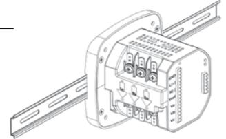
Shark® 100T - DIN Rail Mounted Transducer
